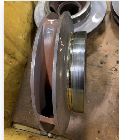
Impeller Wear Ring: Minimal damage after running against dures® XPC-2 case wear ring
