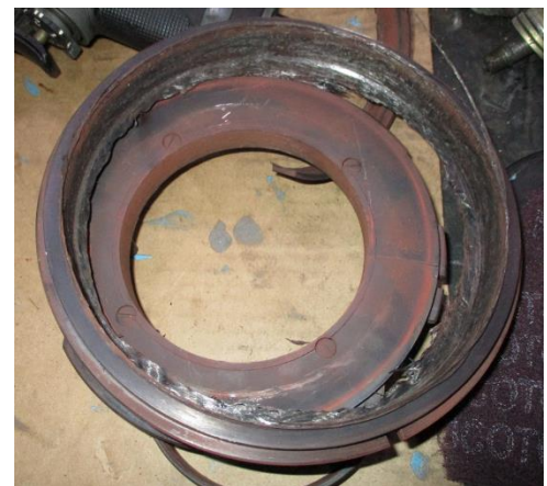
Case Wear Ring: Evidence dures® XPC-2 components acted as sacrificial components protecting the pump from total loss
